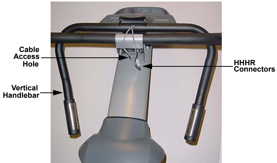
Diagram 7.9 - Vertical Handlebar Removal
