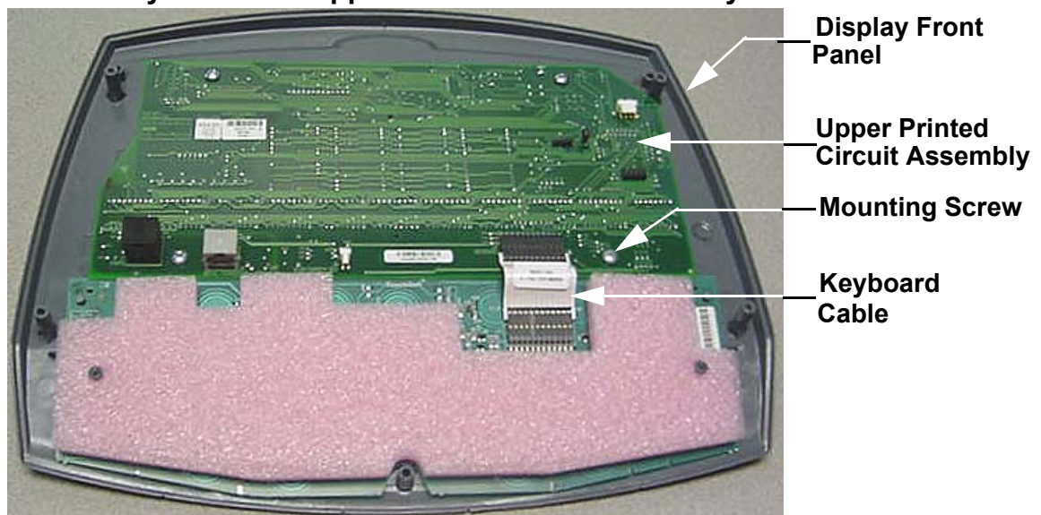
Diagram 7.1 - Keyboard and Upper Printed Circuit Assembly
