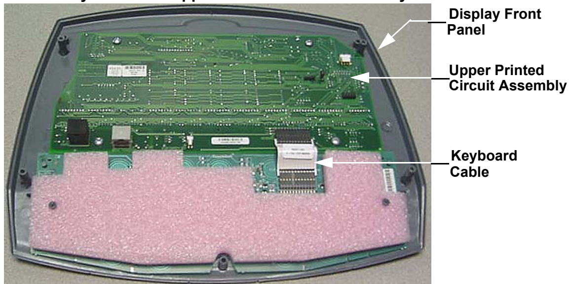
Diagram 6.3 - Keyboard and Upper Printed Circuit Assembly
